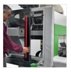
Facilitated access during tool change operations thanks to the openable front
