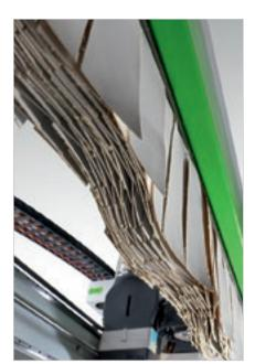
**Side curtain guards** to protect the working unit, which are movable to enable the machine to work at maximum speed in total safety.
