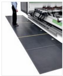
**Pressure-sensitive floor mats** enable the machine to operate at constant maximum speed.
