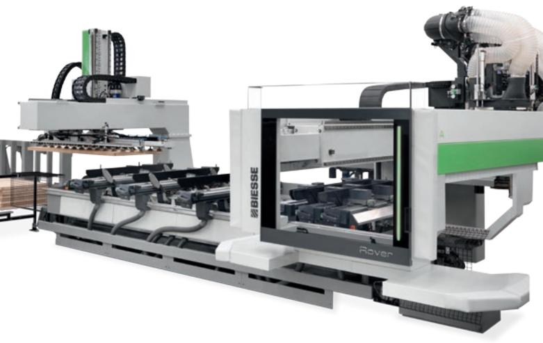
Synchro can also machine stacks of different-sized panels, thanks to stack reference device and the panel pre-alignment cycle, which is performed while the machine is running, while the Rover machining centre processes the previous panel.
